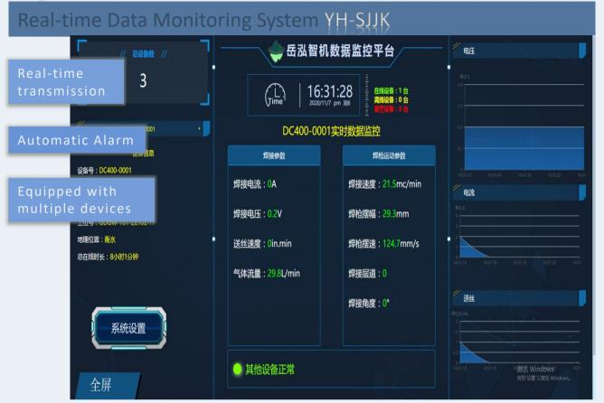
The data monitoring platform includes welding terminal data acquisition system and cloud data intelligent management system.Real-time collection, processingand analysis of on-site welding construction parameters, such as welding current, welding voltage, welding layer information, wire feeding speed and welding speed, etc.
